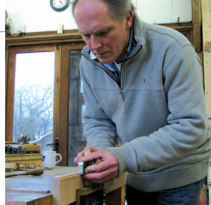
Pic. 17 A shoulder plane can be used for the shoulders of a double tenon on a door rail (above left), and for rebates (above), but beware tearing the grain
