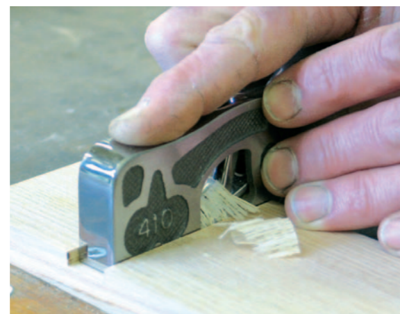
Pic. 16 Shoulder planes can be used across the grain to tickle a rebate (or tenon, left) or to clean up a housing (above). A chisel plane can be used for a stopped housing
