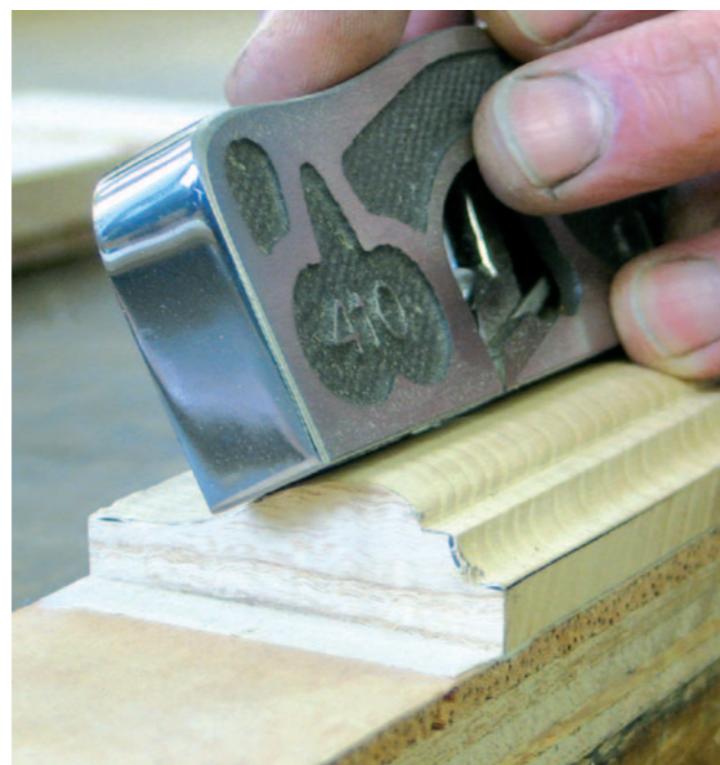
Pic. 18 Because it's quite slim you can get a really good feel with the shoulder plane, using your hands as a fence for rebates (top) and for working on cross-grain mouldings (left). It is for this sort of shaping that Garrett Hack praises the shoulder plane. Sometimes you have to hold the plane in both hands, working across the grain (above)
