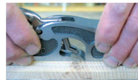
Pic. 18 Because it's quite slim you can get a really good feel with the shoulder plane, using your hands as a fence for rebates (top) and for working on cross-grain mouldings (left). It is for this sort of shaping that Garrett Hack praises the shoulder plane. Sometimes you have to hold the plane in both hands, working across the grain (above)
