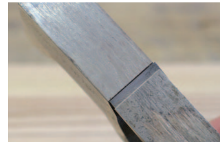
Pic.11 Check that the mouth opening is fine and even. You can see where the plating on John's old 92 has been ground away for a short length behind the blade opening where the sole flexes (bottom right)
