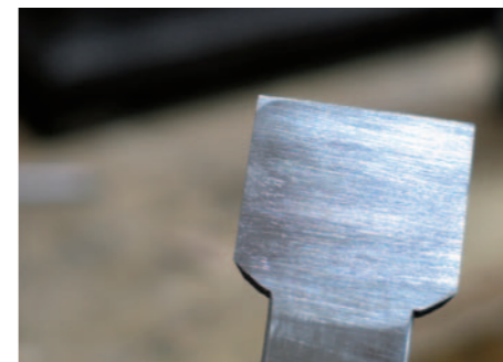
Pic.11 Check that the mouth opening is fine and even. You can see where the plating on John's old 92 has been ground away for a short length behind the blade opening where the sole flexes (bottom right)
