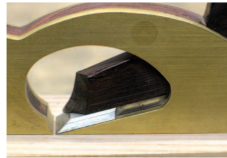
Pic.7 The thin casting on which the blade sits in a shoulder plane can flex. You have to flatten the sole with the blade in position
