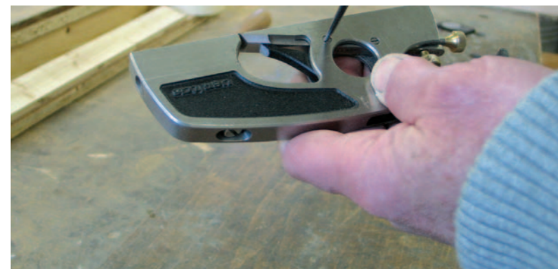
Pic.13 Veritas grub screws can help to position the blade
