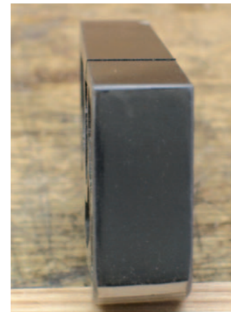
Pic.10 Set the blade up with a fine, even projection by sighting along the sole (see Pic.2)
