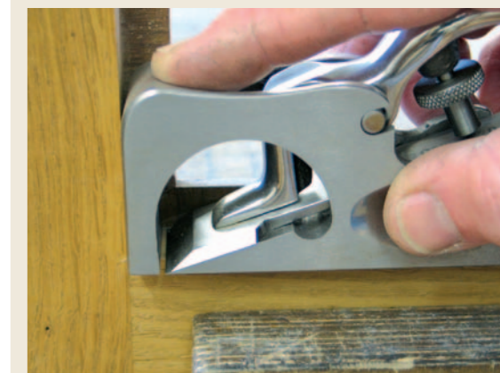
Pic. 17 A shoulder plane can be used for the shoulders of a double tenon on a door rail (above left), and for rebates (above), but beware tearing the grain
