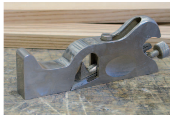
Pic.1 John's first shoulder plane, a rather ordinary Stanley 92, was bought from Thanet Tools in about 1990. He had just started training at Bruce Luckhurst's and a shoulder plane was on the tool list
