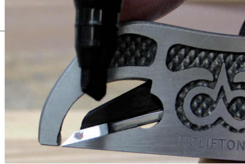
Pic.9 Mark the edge of the blade with a felt tip pen as a reminder when sharpening which side of the blade you need to grind back. There is only a tiny amount of lateral adjustment on a shoulder plane, so the blade has to be ground very accurately. The blade must stick out evenly, and there is very little tolerance
