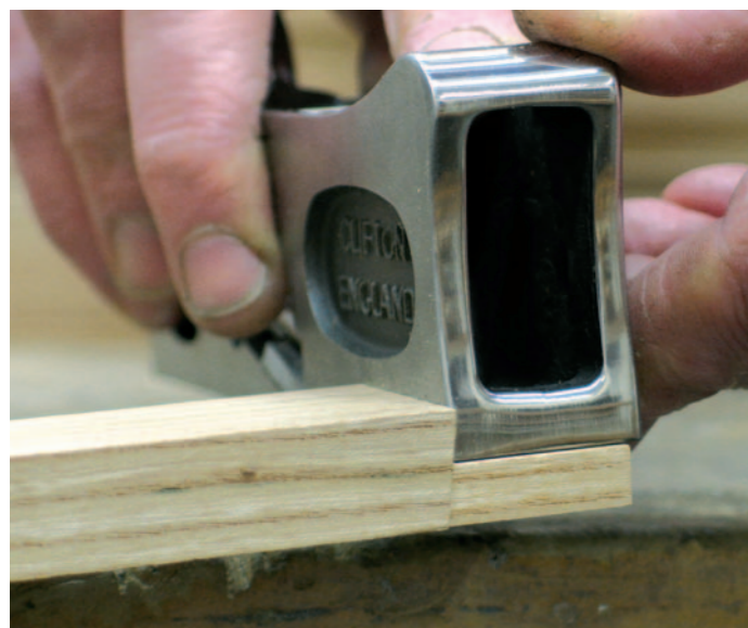
Pic. 16 Shoulder planes can be used across the grain to tickle a rebate (or tenon, left) or to clean up a housing (above). A chisel plane can be used for a stopped housing
