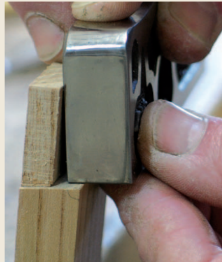
Pic.5 An angled shoulder prevents the use of a shoulder plane
