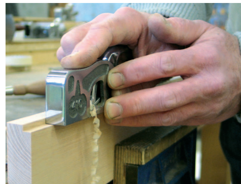
Pic. 17 A shoulder plane can be used for the shoulders of a double tenon on a door rail (above left), and for rebates (above), but beware tearing the grain
