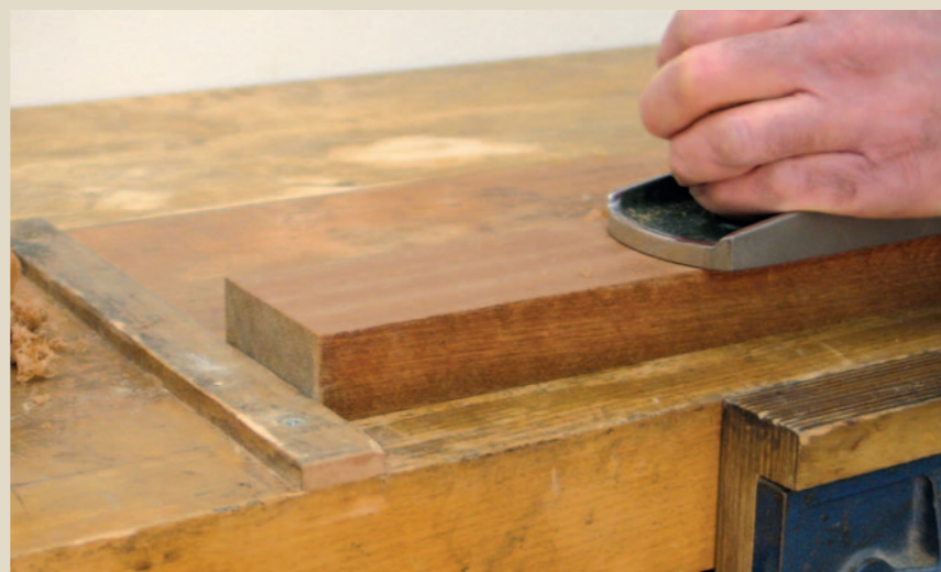
Pic.6 John has made a removable planing stop (top) because he doesn't much care for the toothed and sprung metal versions (above)
