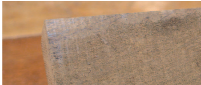
Pic.8 By rubbing the sawn surface on the bench (top) you will identify the high points (above), which take a glazed look. Concentrate on planing these 'hills' until the board will lie flat (right). The paper (below) is used when planing a thin piece of wood that is bowed, but needs to be flattened
