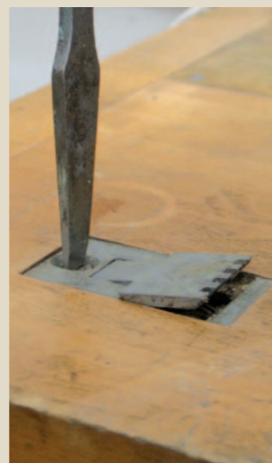
Pic.6 John has made a removable planing stop (top) because he doesn't much care for the toothed and sprung metal versions (above)
