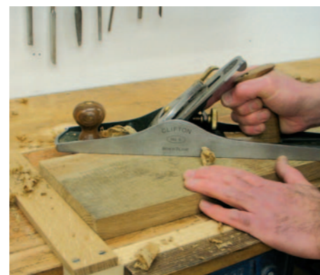
Pic.9 Planing sawn timber against a removable stop. Notice how John is doing this one-handed (left) for speed as the purpose is to flatten the board partially for planing level properly
