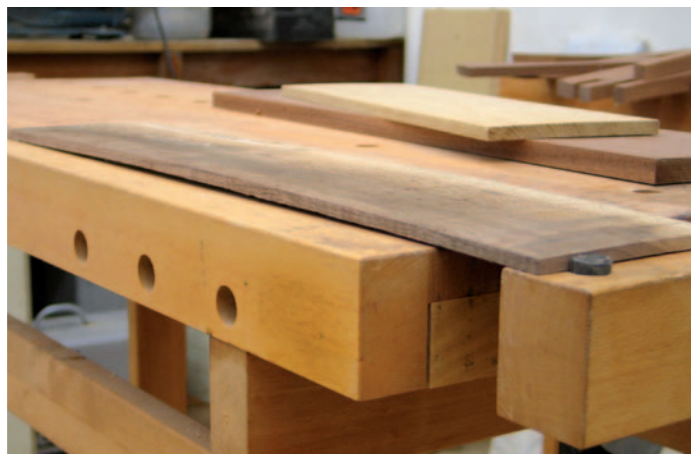
Pic.4 A tail vice can bend thinner boards if over-tightened (above). The tail vice is often not level with the bench top (left)
