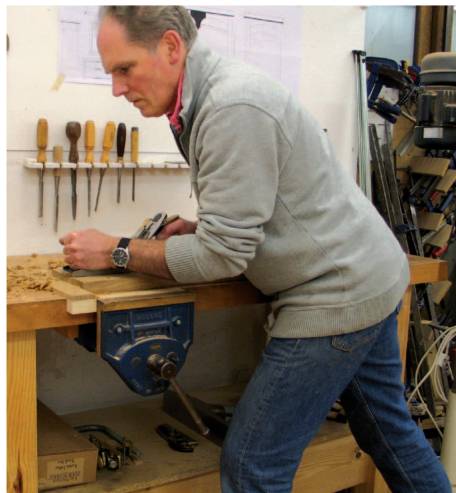
Pic.1 The simple tools you need to hold a board in place for surface planing. The L-shaped stop (far left) fits in the bench vice and can be made with any thickness of arm, to suit the board you are planing. The hold-downs are used with the simple wooden bar (top, above), which stops a board from wiggling around
