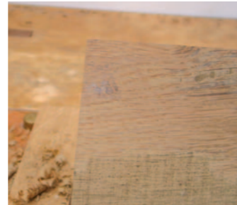
Pic.8 By rubbing the sawn surface on the bench (top) you will identify the high points (above), which take a glazed look. Concentrate on planing these 'hills' until the board will lie flat (right). The paper (below) is used when planing a thin piece of wood that is bowed, but needs to be flattened
