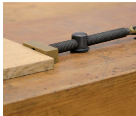
Pic.5 Veritas's Wonder Pups are great for holding thicker pieces, but they are often too tall for surface planing unless you grind them down (left, above)
