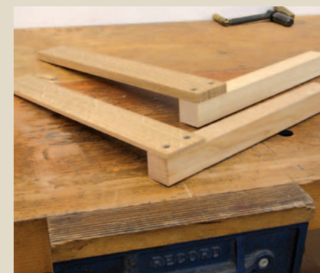
Pic.7 A screwed-down stop is ok (left), but there is a risk you'll plane too energetically and clip one or more of the fixing screws
