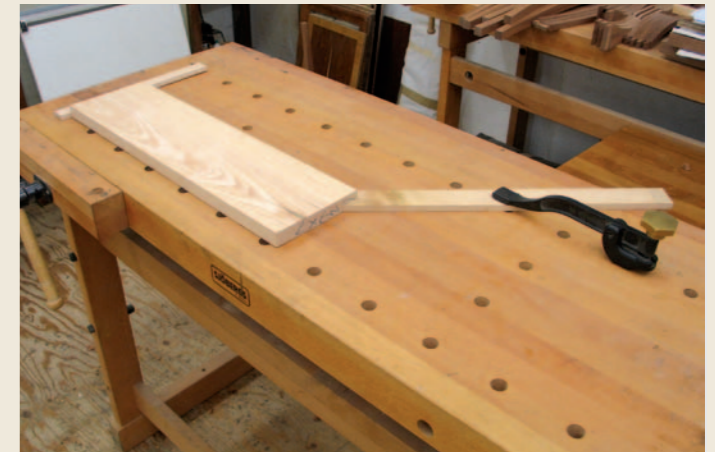
Pic.10 The simplest of stops. A batten between two dogs at the far end and an angled batten with bird's mouth notch at the other
