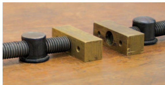
Pic.5 Veritas's Wonder Pups are great for holding thicker pieces, but they are often too tall for surface planing unless you grind them down (left, above)
