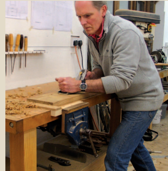
Pic.7 A screwed-down stop is ok (left), but there is a risk you'll plane too energetically and clip one or more of the fixing screws
