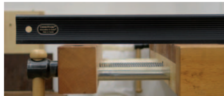
Pic.4 A tail vice can bend thinner boards if over-tightened (above). The tail vice is often not level with the bench top (left)
