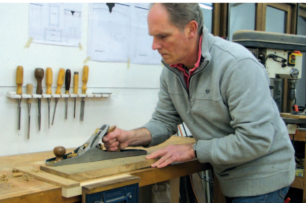
Pic.9 Planing sawn timber against a removable stop. Notice how John is doing this one-handed (left) for speed as the purpose is to flatten the board partially for planing level properly
