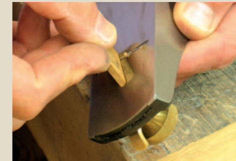
Pic.14 An alternative method for tapering the plug for a tight fit in the cavity is with a block plane (left). Have it set really fine, with the mouth tight too
