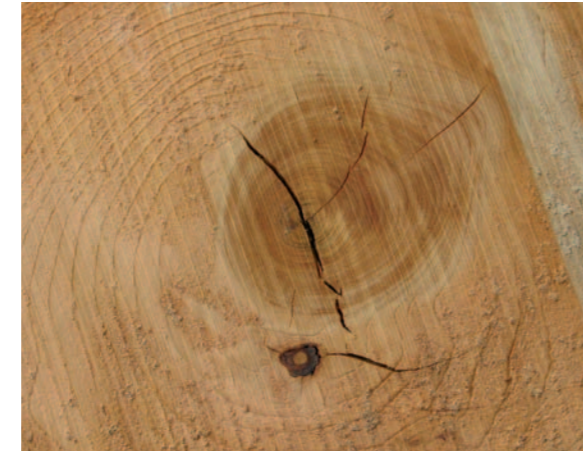
Pic.1 A live knot with a shake. A live knot is stronger than a dead one, and can look perky and healthy
