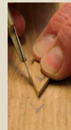
Pic.15 Line the grain direction of the patch on the knot (left) then mark the diamond shape and rout out the bulk of the waste
