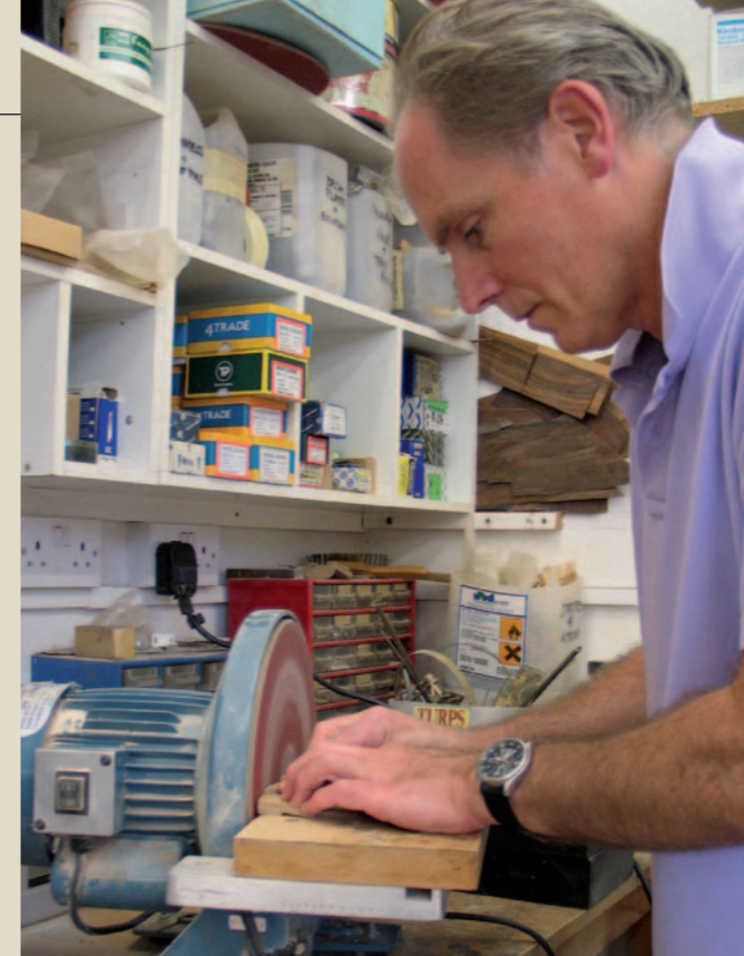
Pic.13 Make sure you mark which direction the grain runs in (left) before cutting out the patch and tapering it to shape on a disc sander (above)
