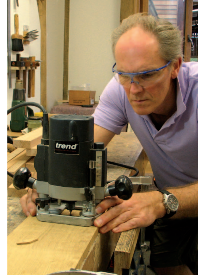
Pic.6 You can rout to a line with a fine cutter freehand quite easily to remove a knot
