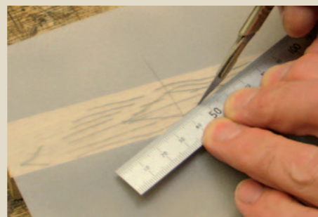
Pic.12 If you want to completely 'lose' a knot you will need to make a diamond patch. Trace around the knot and add grain lines (above). Then cut through the tracing paper onto the wood that is going to be a patch
