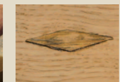
Pic.17 The patch should be slightly proud (above) then planed level
