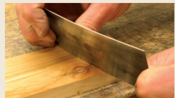
Pic.9 Pare the excess epoxy back with a chisel (left), then level with a scraper (above) before adding any necessary acrylic colour with a fine brush (right). Finished (top)!
