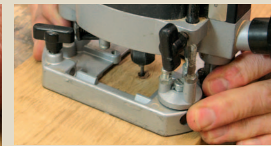
Pic.15 Line the grain direction of the patch on the knot (left) then mark the diamond shape and rout out the bulk of the waste
