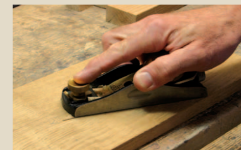
Pic.17 The patch should be slightly proud (above) then planed level
