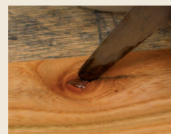
Pic.8 Use a palette knife to push the mixed epoxy into the knot. Leave the epoxy proud
