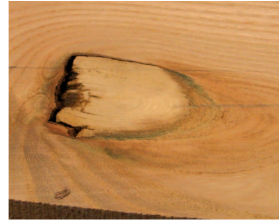
Pic.4 On the other side of Pic.3, however, is a much more dangerous-looking semi-dead knot ready to chip away
