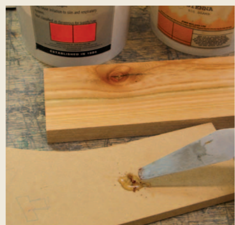
Pic.8 Use a palette knife to push the mixed epoxy into the knot. Leave the epoxy proud
