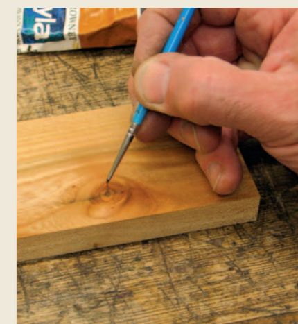
Pic.9 Pare the excess epoxy back with a chisel (left), then level with a scraper (above) before adding any necessary acrylic colour with a fine brush (right). Finished (top)!
