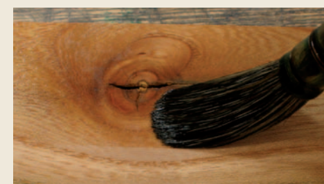
Pic.7 Brush shellac on the knot so that the epoxy doesn't contaminate the grain, then mix the epoxy with pigment (right)
