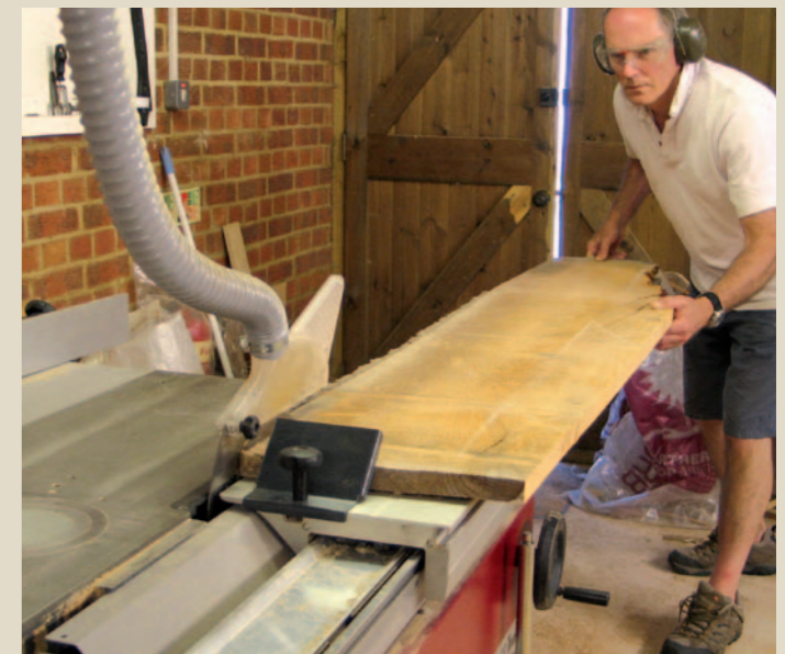
Shoes Using the shoe on a Hammer tablesaw to hold a board while ripping it. John has an old Chalk-O-Matic chalk line to mark out quick straight edges
