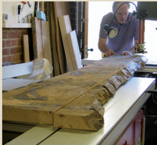
Bandsaw The challenge with a bandsaw is supporting the end as it comes off the table. Fortunately John's tablesaw is the same height, but you may prefer to use roller stands
