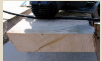
Skill Remove any shakes at the end of a board with a Skil saw, but otherwise a board like this will be ripped in two
