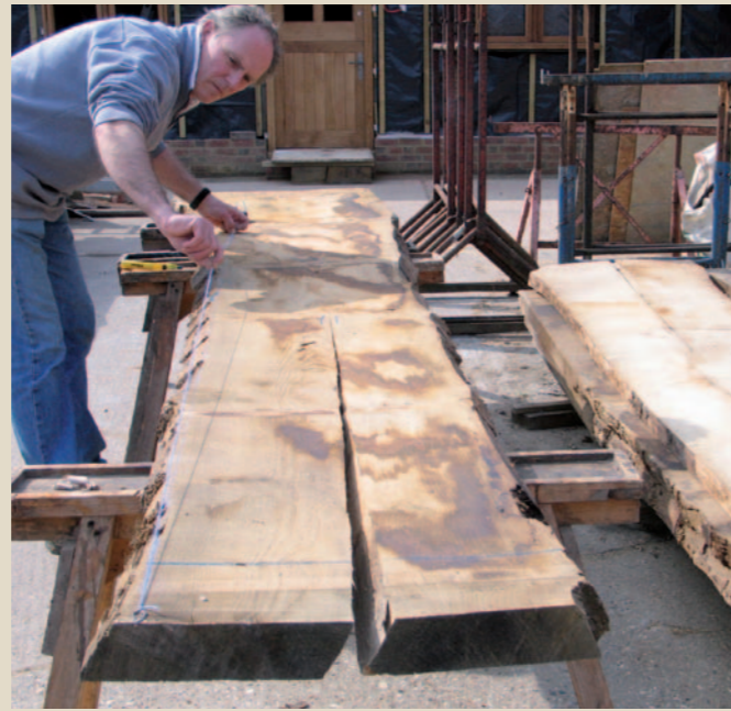
Snappy John using a chalk line to mark the straight edge along the waney-edged board. If there is a lot of curve consider cutting the board in two so there is less waste
