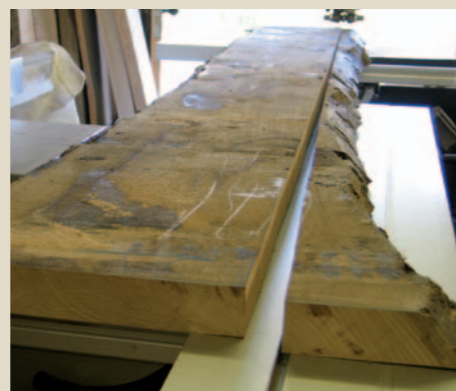
Bandsaw The challenge with a bandsaw is supporting the end as it comes off the table. Fortunately John's tablesaw is the same height, but you may prefer to use roller stands
