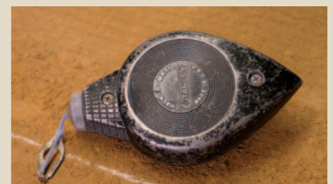
Shoes Using the shoe on a Hammer tablesaw to hold a board while ripping it. John has an old Chalk-O-Matic chalk line to mark out quick straight edges
