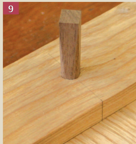
Taper Pare back the square peg to fit it into a round hole. It's a good idea to pare the end of the round peg too to help it into the hole and through the joint
