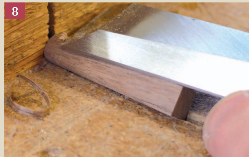
Taper Pare back the square peg to fit it into a round hole. It's a good idea to pare the end of the round peg too to help it into the hole and through the joint
