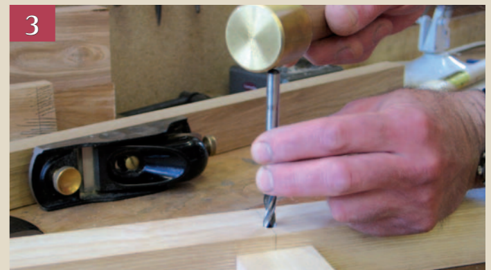
Marking Use the drill bit to mark the position for the hole in the tenon. Timber framers have special offset markers for this job
