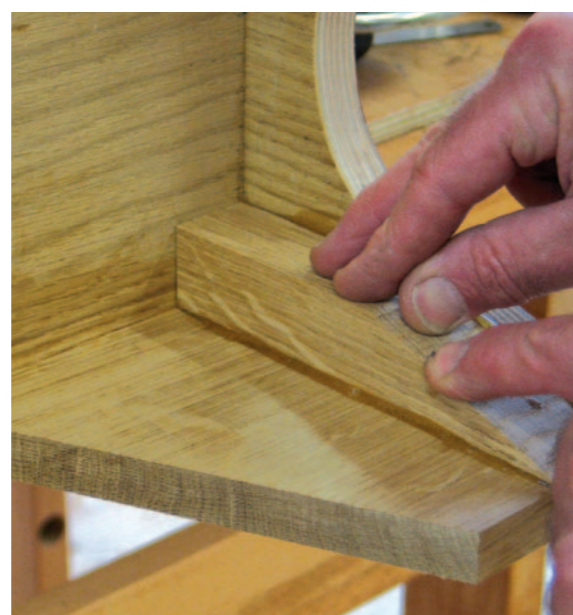
Rubbing The traditional rub joint with animal glue being used on bracket feet (above and top right) and for the apron of a table (above right). Spreading PVA to attempt a rub joint with modern glue (right)
