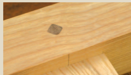
Pegs The finished joints, with a round (above left) and a square peg (left). The latter is particularly decorative
