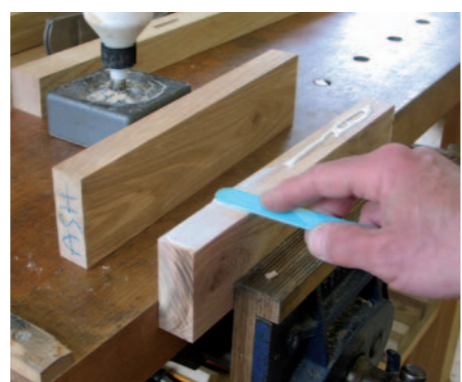
Rubbing The traditional rub joint with animal glue being used on bracket feet (above and top right) and for the apron of a table (above right). Spreading PVA to attempt a rub joint with modern glue (right)
