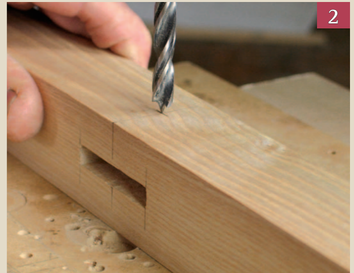
Spurred Use a lip and spur bit to drill the hole through the mortise. You can insert a false tenon to reduce breakout inside the mortise
