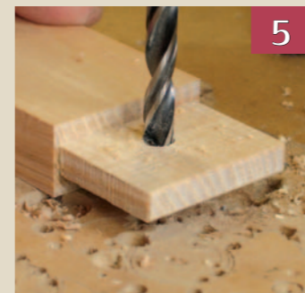
Offset Having established the offset on the tenon you drill through for the peg, which will have to wiggle its way through
