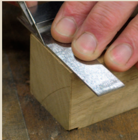
Scribe One way to reduce tearout is to scribe a line around the workpiece with a knife (left), and work back from that
