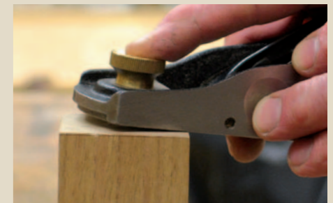
Options Planing towards an end stop is a popular way of avoiding tearout (top). Or you can work towards the centre (above)
