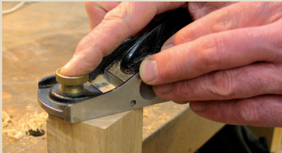
Smooth Whatever method you choose, the iron has to be very sharp to leave end grain smooth
