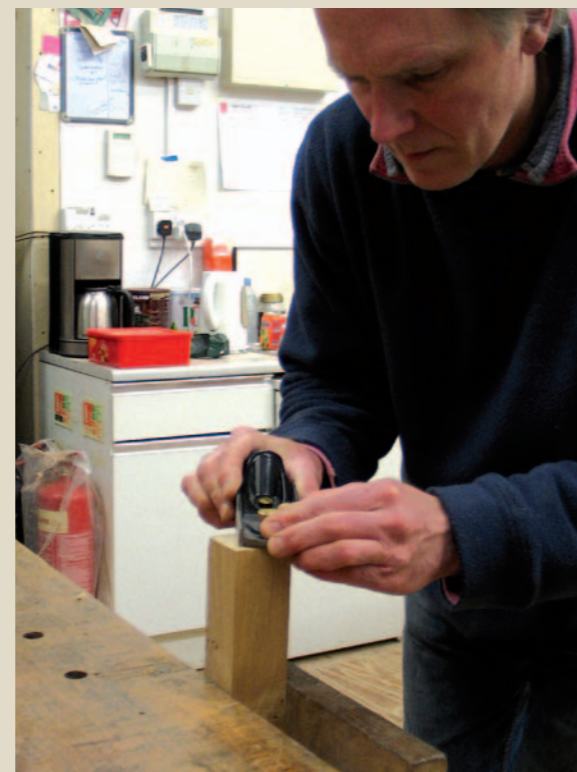
Smooth Whatever method you choose, the iron has to be very sharp to leave end grain smooth
