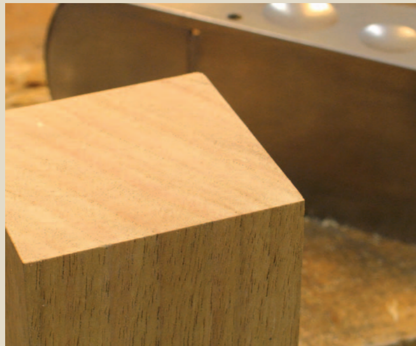
Smooth Whatever method you choose, the iron has to be very sharp to leave end grain smooth
