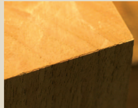
Scribe One way to reduce tearout is to scribe a line around the workpiece with a knife (left), and work back from that
