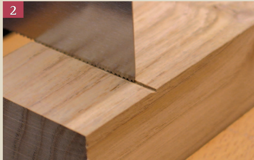
Pics.2&3 The saw sits in the chiselled V, without damaging the vital shoulder line (above). Cut the whole way down the shoulder to the cheek (right)
