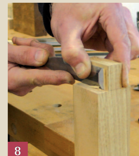
Pics.6&7 Complete the cut down to the shoulder (above) and then tidy up the junction between the shoulder and the cheek with a sharp (of course) chisel (right)
