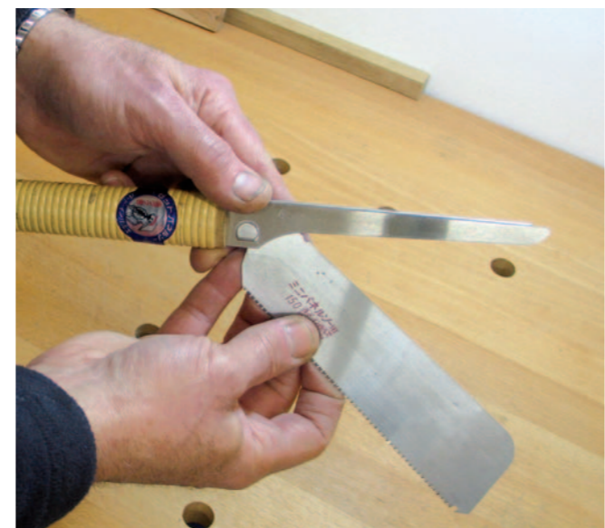
Pic.2 Various styles of Japanese saw. In the centre is the double-bladed Ryoba-Dozuki, with its rip and crosscut teeth, and its depth setting
