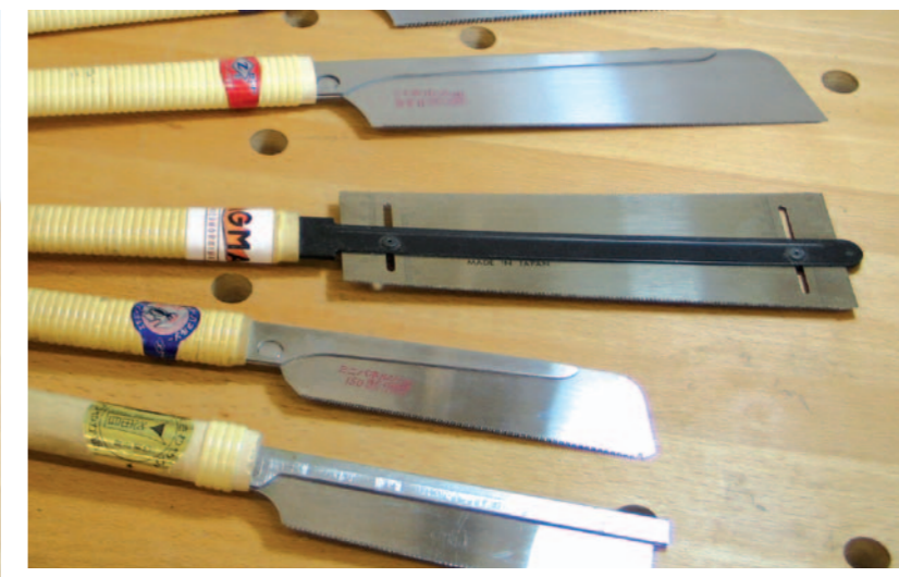
Pic.2 Various styles of Japanese saw. In the centre is the double-bladed Ryoba-Dozuki, with its rip and crosscut teeth, and its depth setting
