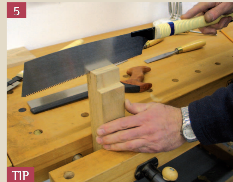
Pic.5 John only cuts one diagonal before sawing straight down the cheek (above). He says the blade is more stable that way
