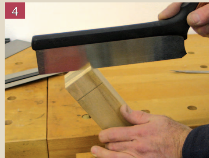
Pic.4 For Western saws the rail needs to be angled away from you, but towards you for Japanese saws (left)
