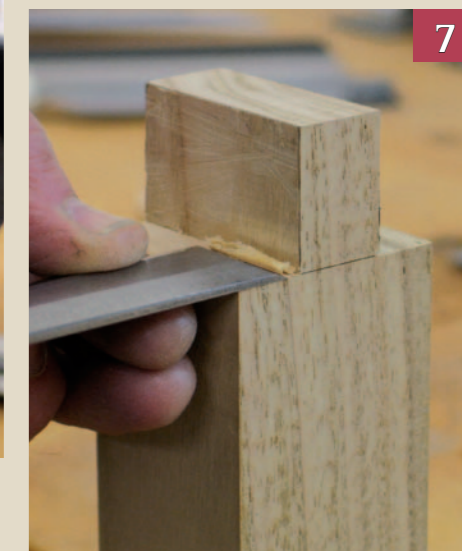
Pic.5 John only cuts one diagonal before sawing straight down the cheek (above). He says the blade is more stable that way
