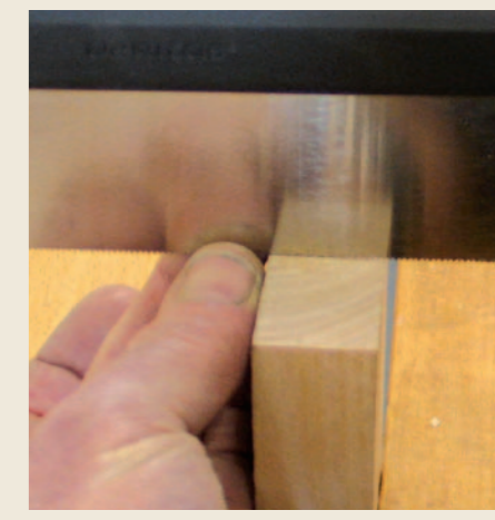
Pic.4 By pinching with thumb and index finger you get better control at the start, but beware the risks of injury!
