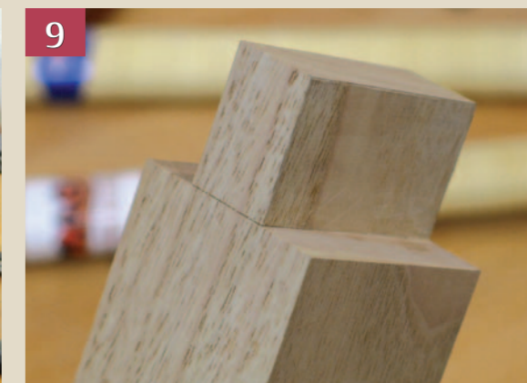
Pics.8&9 Tidy up paring across the cheek and you should have a perfect tenon ready for fitting
