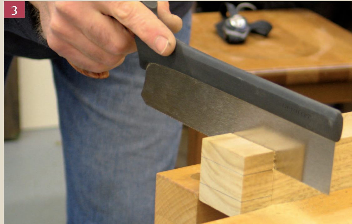
Pics.2&3 The saw sits in the chiselled V, without damaging the vital shoulder line (above). Cut the whole way down the shoulder to the cheek (right)
