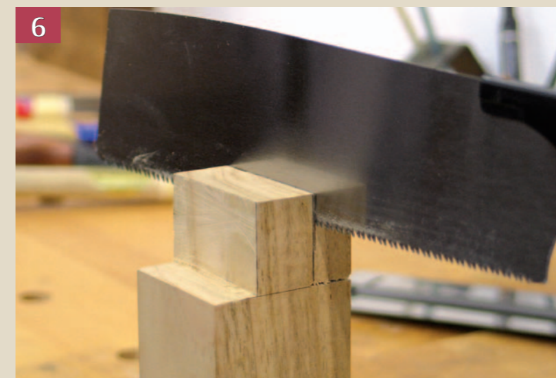
Pics.6&7 Complete the cut down to the shoulder (above) and then tidy up the junction between the shoulder and the cheek with a sharp (of course) chisel (right)
