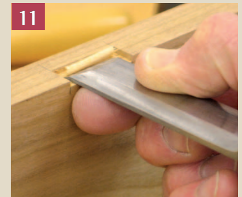
Pic.11 Make final cuts to the gauge line
