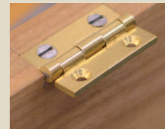
Tidy The completed hinge, with the leaf level to the top and pivot point central
