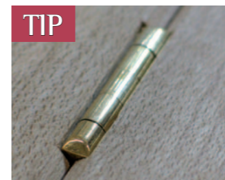
TIP Softer A chamfer filed on the end of a butt hinge softens the knuckle, as suggested by one of John's students, Ian Parker
