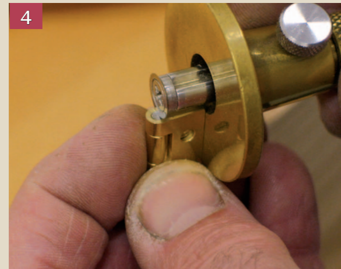
Pic.4 Set the cutting gauge to a little less than the distance from the edge of the leaf to the centre of the pin
