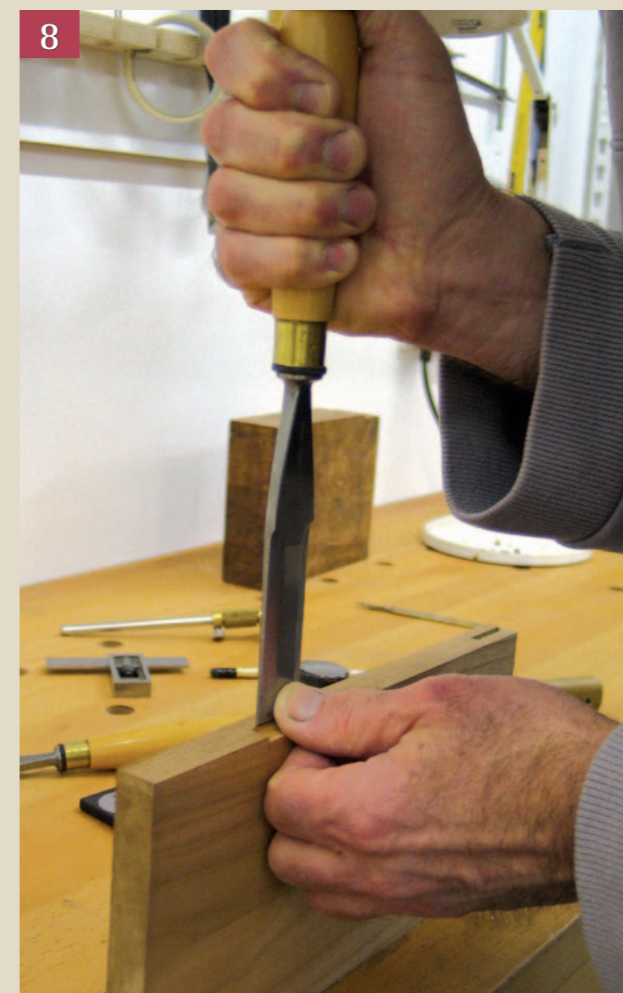
Pic.8 Chop down into the mortice to define the edges of the recess
