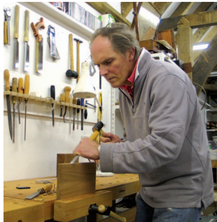
Caring Show that you care by lining up the slotted screws on your hinges. Someone will notice, and so will you! John chops out a hinge recess (or mortice) by hand
