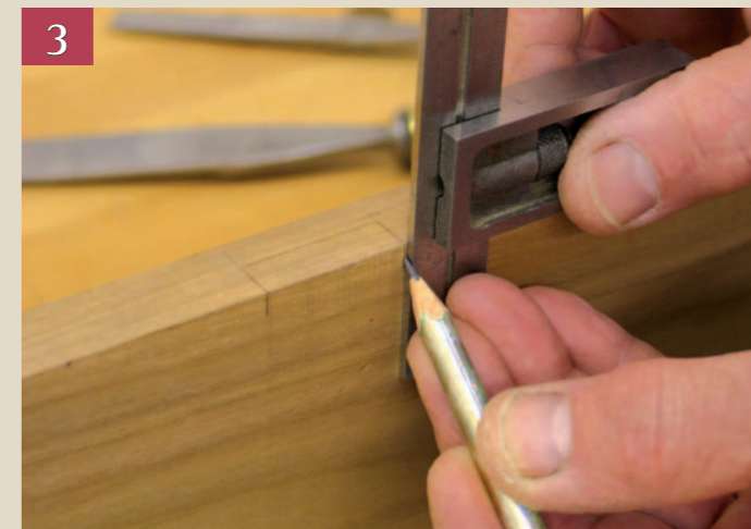
Pic.2 Extend the knife marks with a pencil and square on the face (above) and edge (Pic.3 below) of the workpiece
