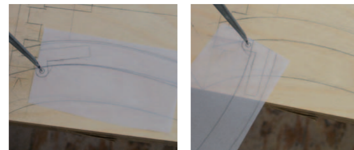
Trick The tracing paper trick from Joyce, with the door closed (left) and open (right). In this case we're testing if the door will open without binding on the carcass, and the drawers won't hit the door
