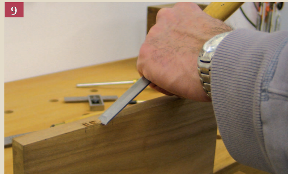
Pic.8 Chop down into the mortice to define the edges of the recess
