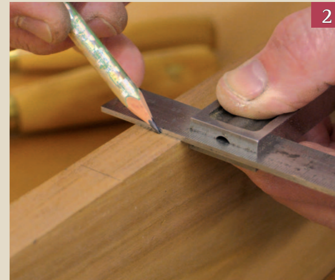
Pic.2 Extend the knife marks with a pencil and square on the face (above) and edge (Pic.3 below) of the workpiece
