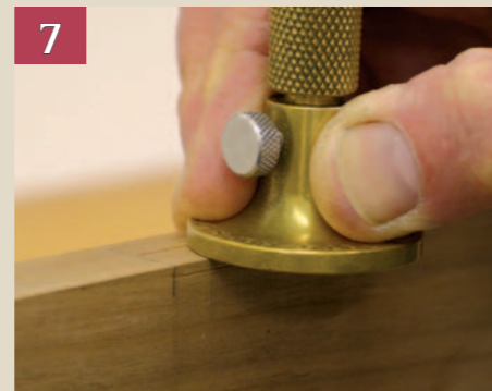
Pic.7 Gauge the depth of the hinge mortice on the face of the rail/stile
