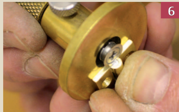
Pic.6 Set the gauge to the thickness of the leaf, or a little less than the face of the leaf to the pin centre
