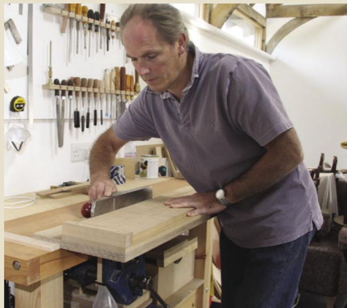
Comfort Many people automatically use a long-grain shooting board as if planing normally (below), but this means reaching over the bench and isn't as comfortable as working 'left-handed' (above)
