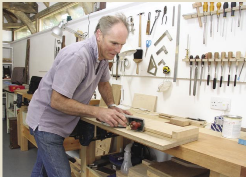
Comfort Many people automatically use a long-grain shooting board as if planing normally (below), but this means reaching over the bench and isn't as comfortable as working 'left-handed' (above)
