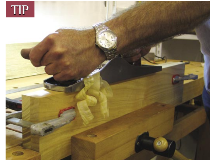
Paired By cramping two pieces together, any discrepancy is nullified when the pieces meet
