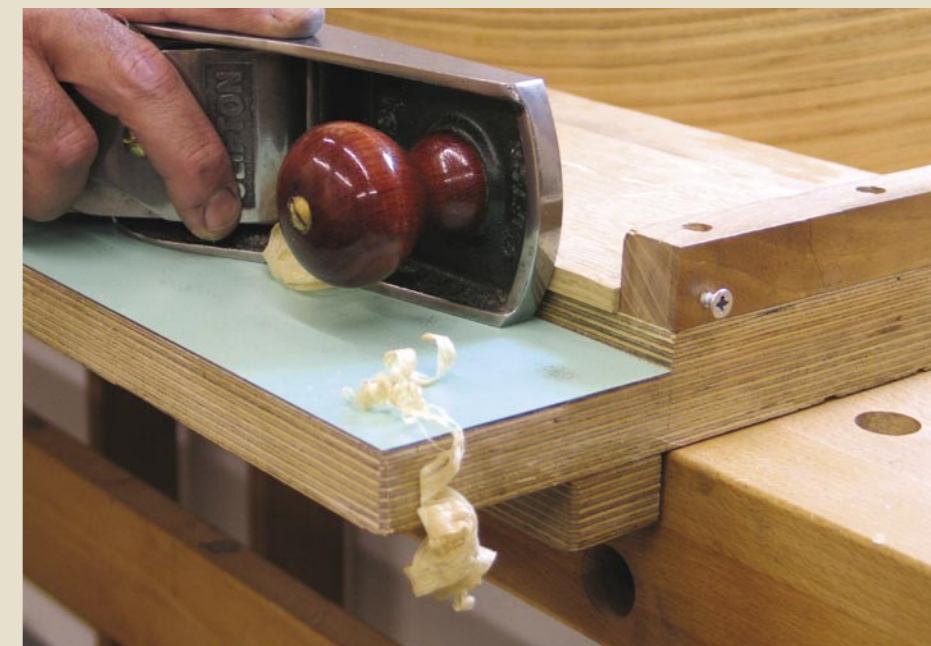
Caul Use a piece of MDF to hold down the Formica either in a vacuum press or with lots of G-cramps
