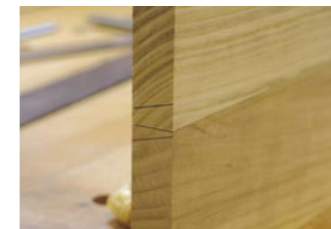
Paired By cramping two pieces together, any discrepancy is nullified when the pieces meet
