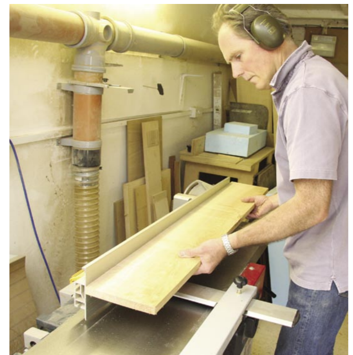
Machining John uses the fence on his planer to check an edge for straightness, but rarely joints edges straight from the planer
