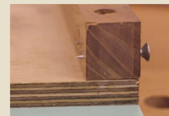
Pin The screw stops the workpiece wandering around. It can be removed to be sharpened or replaced, and can be tuned if you need it longer or shorter
