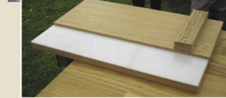
Inspired The addition of a Formica surface to John's MkII shooting board was inspired by Phil Edwards' shooting board at the Festival of the Tree. The Formica is stuck down with PVA
