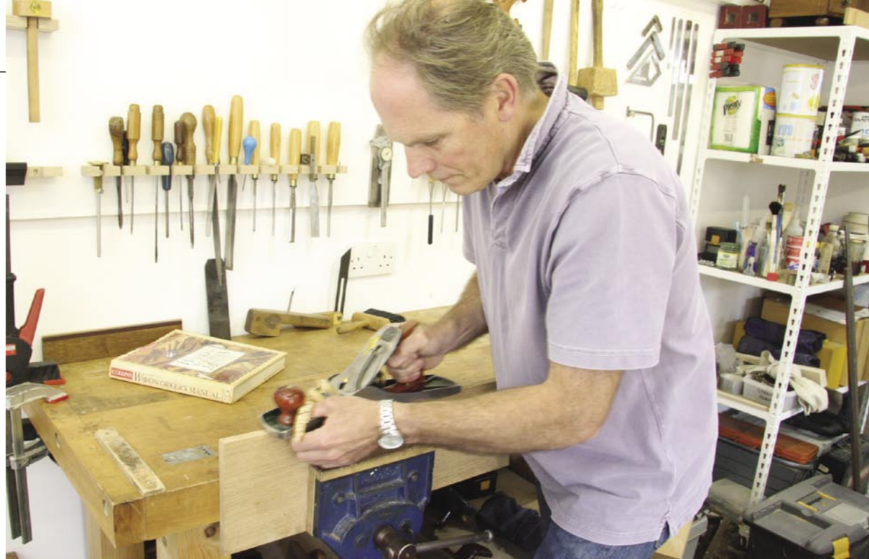
Handwork The initial reason for planing a machined edge by hand is to remove the ripples (left). Planing an edge by machine can at least get the edge straight and give you an edge square to a face
