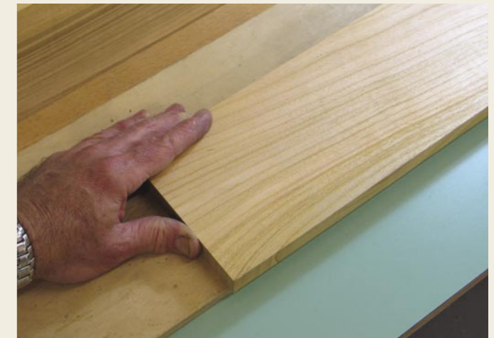
A traditional way that I was shown, to plane a square, straight edge on relatively thin pieces of wood involves a shooting board and a No.5, 5½ or 6 bench plane. The piece of wood that is to be 'shot' is placed on the shooting board, 'face-side' down, with what is to become its 'face-edge' hanging over the edge of the shooting board. The edge of the top part of the shooting board is not used to guide the plane, its only function is to lift the workpiece up enough to make contact with the plane's blade.
