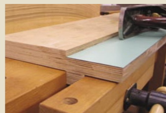
Guide John doesn't use the shooting board to guide the plane, other than keeping it square to the edge. He will either plane to a gauged line or follow the traditional technique (see p51) of hollowing the edge first and then making two or three full passes
