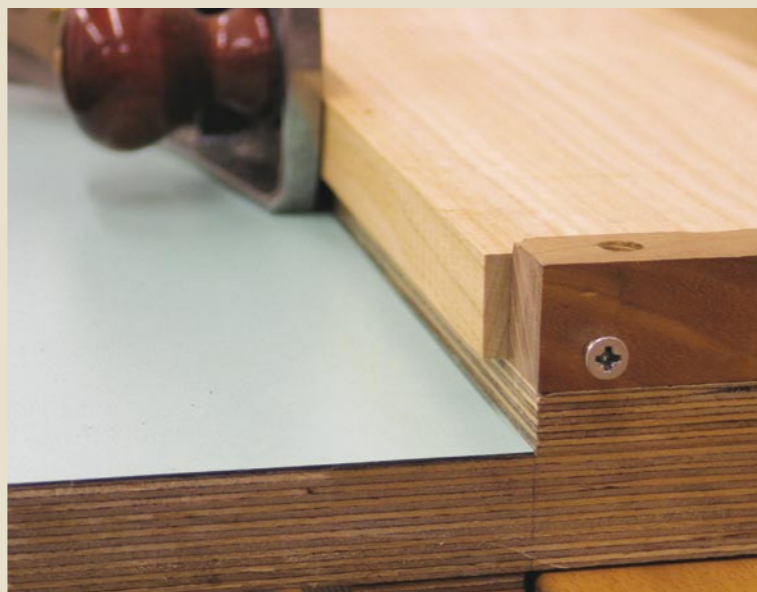
Guide John doesn't use the shooting board to guide the plane, other than keeping it square to the edge. He will either plane to a gauged line or follow the traditional technique (see p51) of hollowing the edge first and then making two or three full passes
