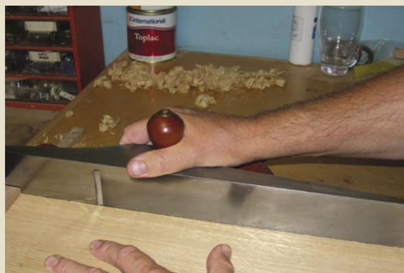
Clifton A friend of John's has a Clifton plane with added knob on the side for use on a shooting board
