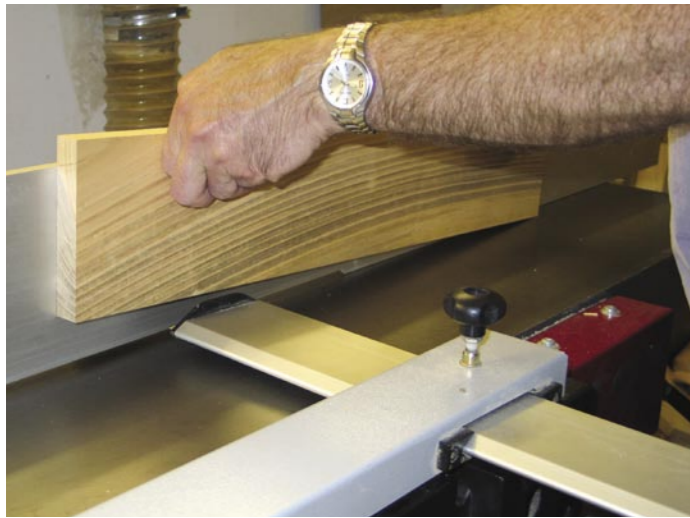
Concave It is possible to plane a concave edge on a planer with a stopped pass, however awkward and dangerous it might feel, but the benefits are negligible as the surface will be bumpy
