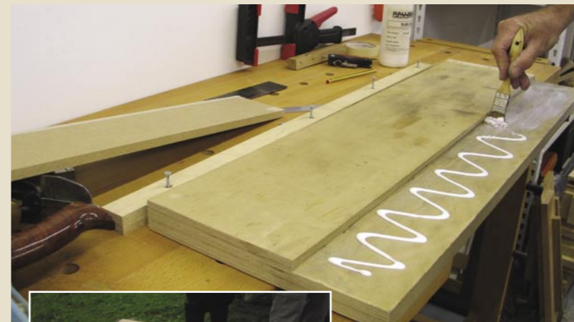
Inspired The addition of a Formica surface to John's MkII shooting board was inspired by Phil Edwards' shooting board at the Festival of the Tree. The Formica is stuck down with PVA
