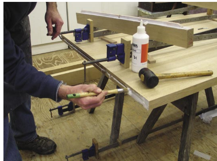
Creep Choosing the right glue is critical when it comes to cleating
