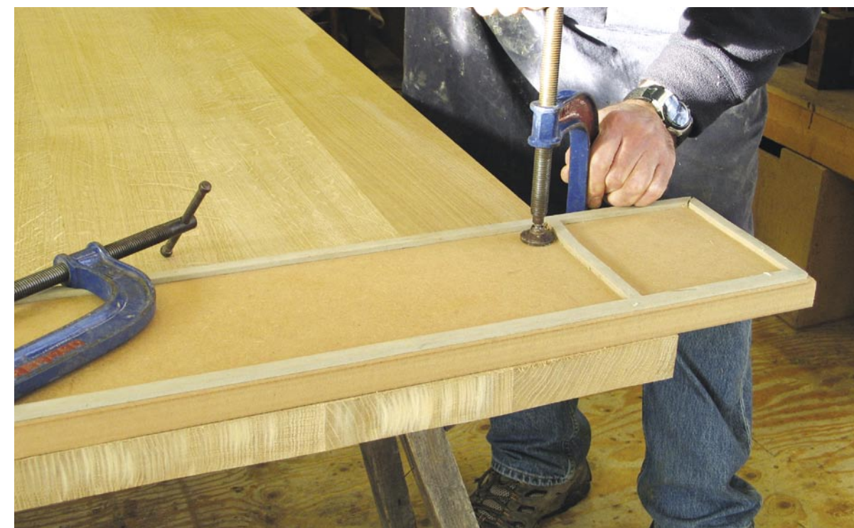
Heavy John favours MDF for straight-edges because it is smooth. He's made his own vacuum edge (below)
