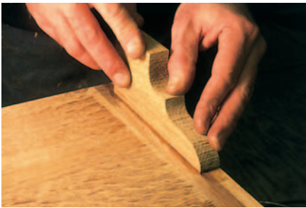
Bracket foot – gluing sequence using rub joints
