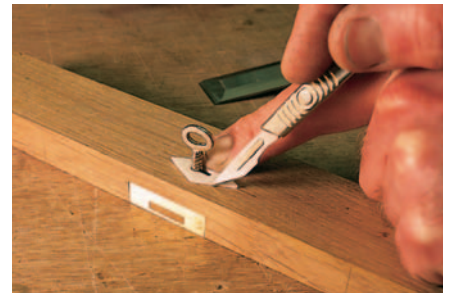
Scribing around edges of escutcheon without removing fingertips!
