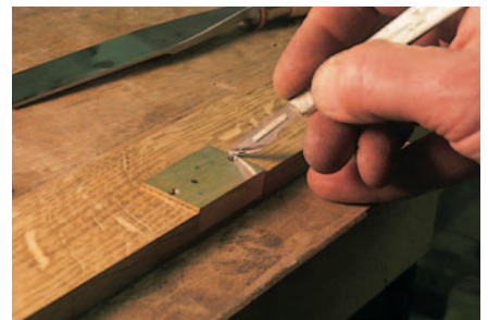
Fitting lock – scribe long side of lock plate
