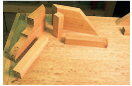
Component parts for bracket feet, no metalwork required, only some Scotch glue
