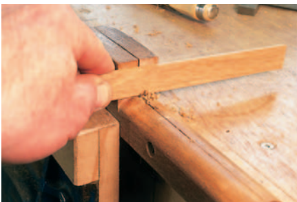
Creating the rounded edge of the cock beading using a scratch-stock and cutter, held in a vice
