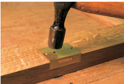
Fitting lock. Mark position of pin by striking outside end of pin with hammer
