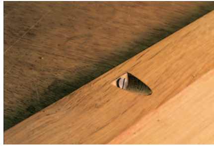
Finished screw pocket, with screw fitted
