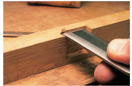
Fitting lock. Scribe edges of lock plate on short side and remove waste
