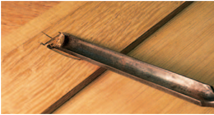
Screw pockets used to secure top to sides – formed using a scribing pattern or ‘incannelled’ gouge, which has the bevel ground on the inside of the curve
