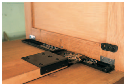
Hafele pocket slide mechanism to make the dummy drawer front 'disappear'
