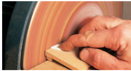
Creating diamond escutcheon using disc sander and angled jig to give slight angle to edges in an attempt to create a perfect fit with no glue lines
