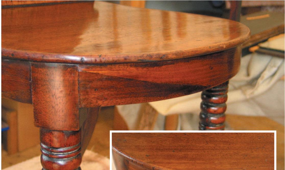
Above: How not to do a veneer repair – the cut is too vertical and the grain direction is bad, causing it to be even more obvious in reflected light
