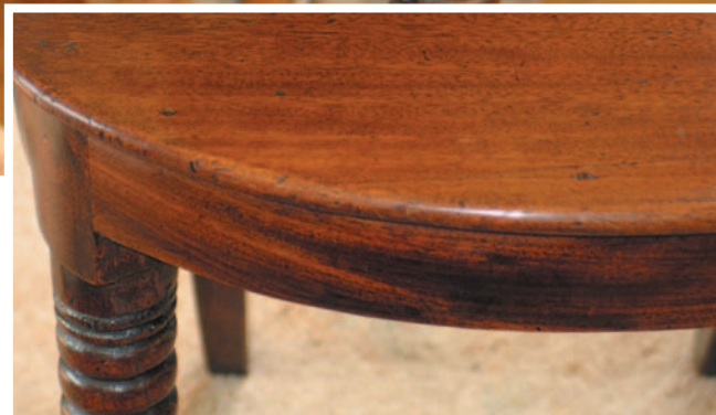
Above: How not to do a veneer repair – the cut is too vertical and the grain direction is bad, causing it to be even more obvious in reflected light
