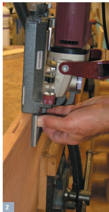
Having created the basic components for the main part of the tool cabinet from birch plywood – see *F&C 93* – it's time to add a bit of lipping to the edges of the ply.
