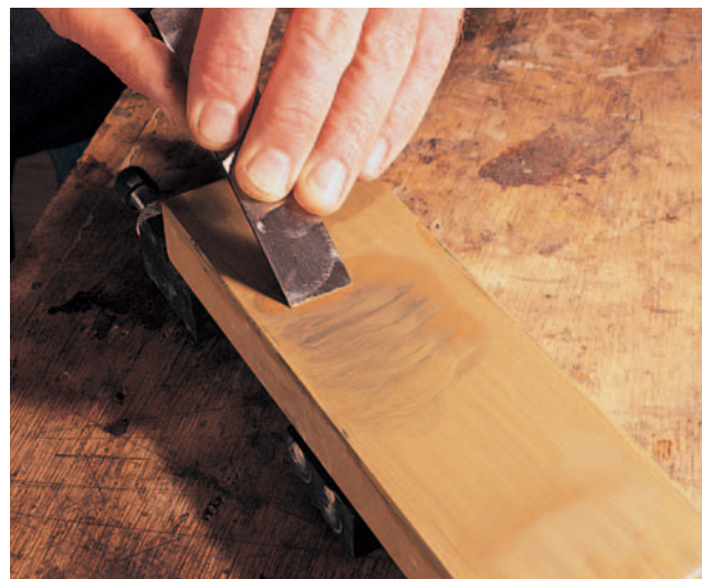
Burnishing bevel on 6000-grit water stone
