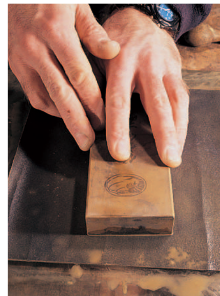
Flattening 6000-grit water stone using 220 wet and dry stuck to a piece of glass and lubricated with water
