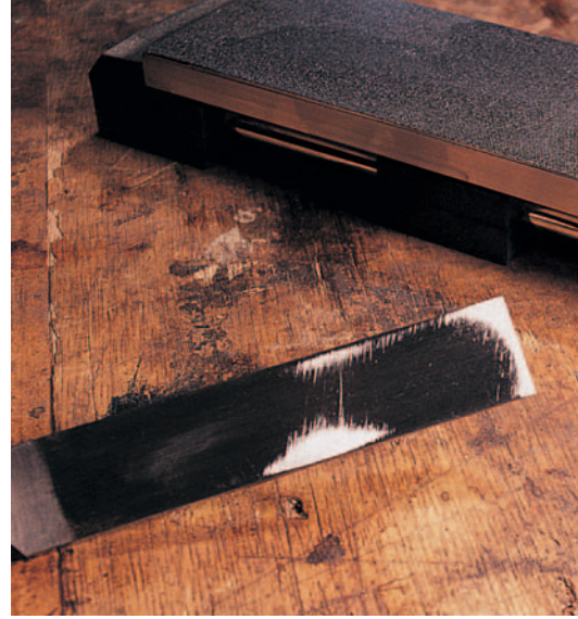
Chisel back showing grinding marks. Achieving flatness in the area of the blade behind the edge is the critical bit; the slightly concave area behind the ground area will reduce with subsequent sharpenings
