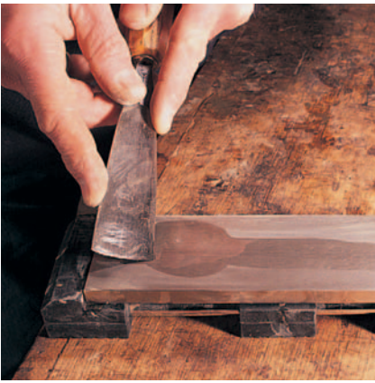
When honing the bevel of the carving chisel, move the chisel from side to side along the stone while turning the chisel and holding it at an angle of 25° and at right angles to the stone – this makes patting your head while rubbing your tummy seem ridiculously simple
