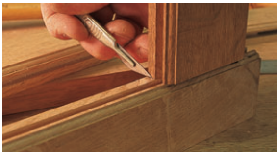
Right: Cutting mitre using jig (top/bottom rail joint)
