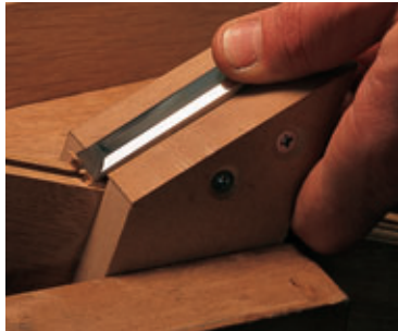
Right: Cutting mitre using jig (top/bottom rail joint)
