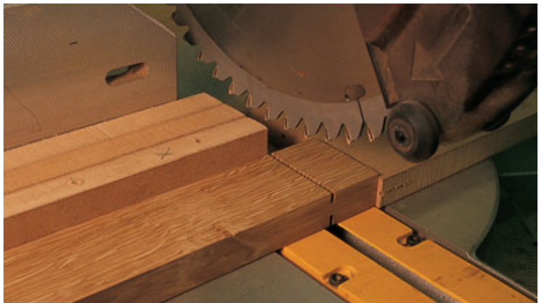
Right: Cutting mitre using jig (mid rail joint)
