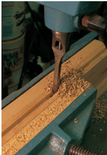
Left: Cutting 6mm mortices centred on groove
