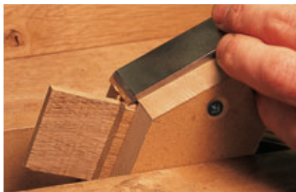
Right: Cutting mitre using jig (mid rail joint)
