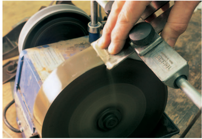
Grinding on a wet stone is the best way to ensure that you don't lose the temper of your steel
