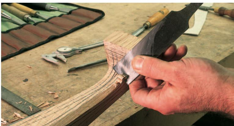
The tighter curves can be shaped with a carving or flat chisel
