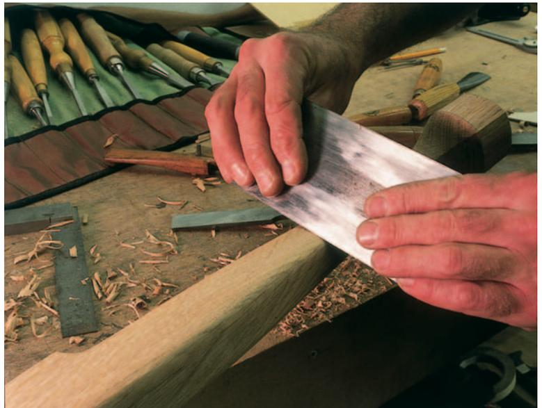
Right: A cabinet scraper is used for final shaping
