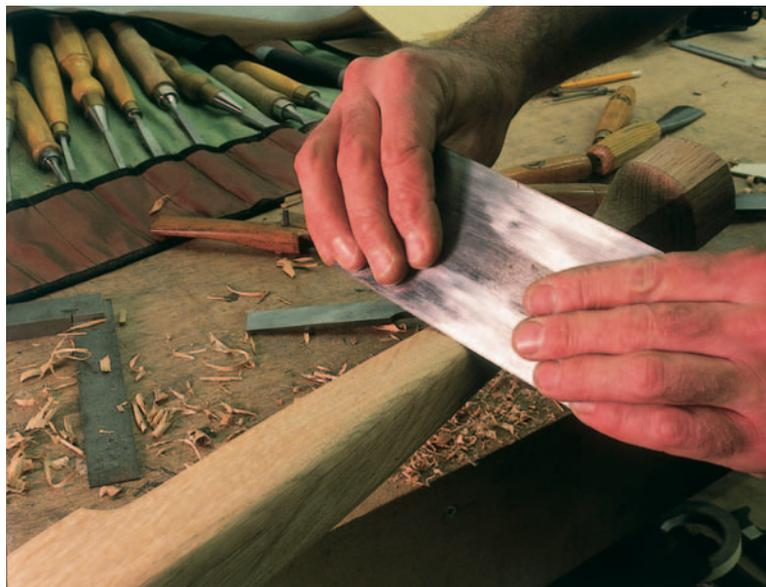
Right: A cabinet scraper is used for final shaping
