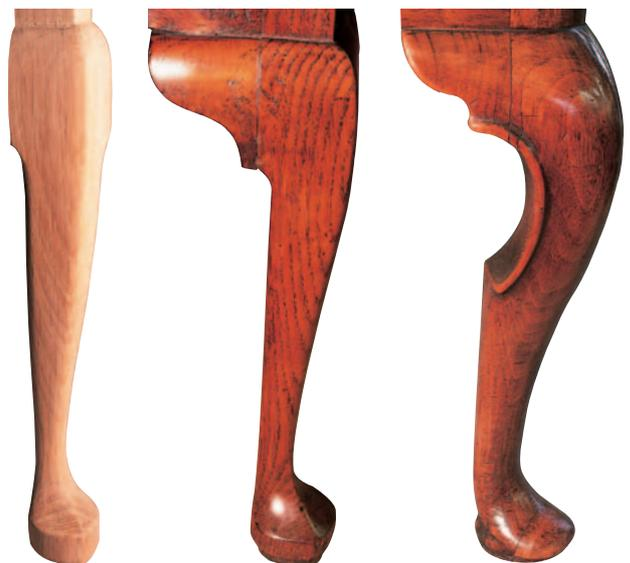
final shaping is done in situ to ensure that the leg curves flow into the ears.
