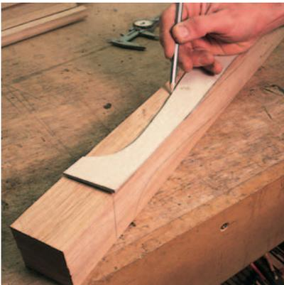
Having made your template from thin ply or cardboard, transfer it to the leg blank
